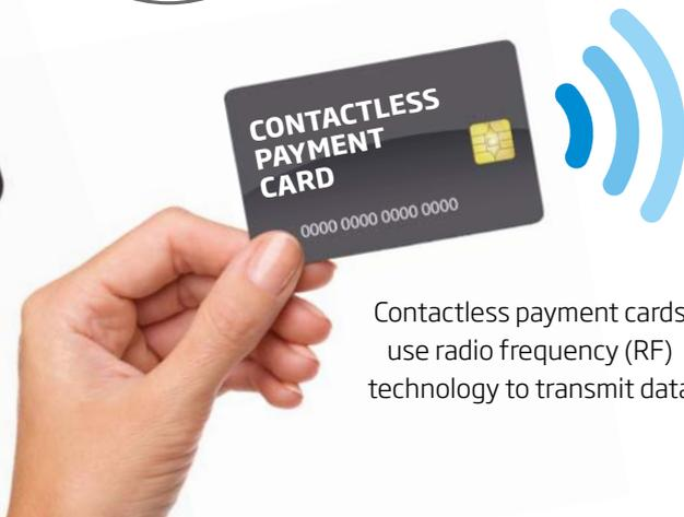
Contactless payment cards use radio frequency (RF) technology to transmit data
