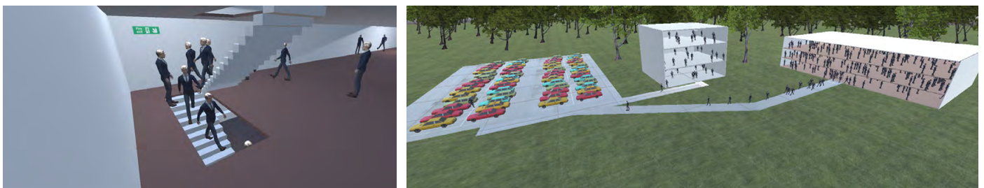
Figure 8: Example simulation (represented within the WUI-NITY model) of people evacuating downstairs and then transitioning from pedestrian to vehicle movement from a multi-occupancy location (Source: Ronchi et al (2017), Wahlqvist et al (2020)).
