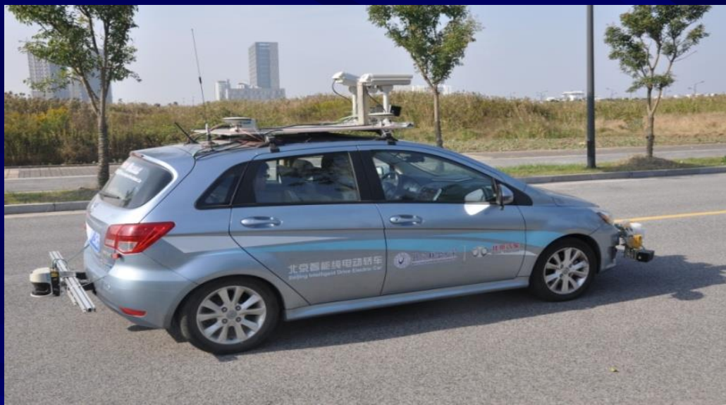
Jing Long No. 1, Jing Long No. 2: the self-driving vehicles developed by intelligent driving team of Beijing Union University on the basis of BAIC MOTOR C70 car and BAIC MOTOR EV150 pure electric car, achieved excellent grades in China Intelligent Vehicle Future Challenge from 2014 to 2016, and broadcast live on CCTV news for many times.
