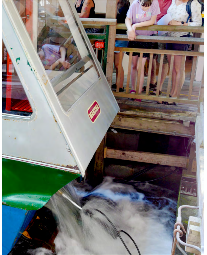
Water is discharged by the car at the bottom of the track – soon it will be pulled up to the top with its load of passengers.
