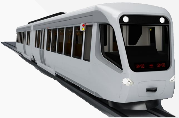
LRT Palembang Aluminum construction
