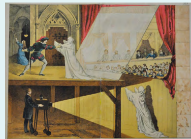
Stage setup for Pepper's Ghost during a theatre show. To the audience, it appears as if the ghost is on stage.
