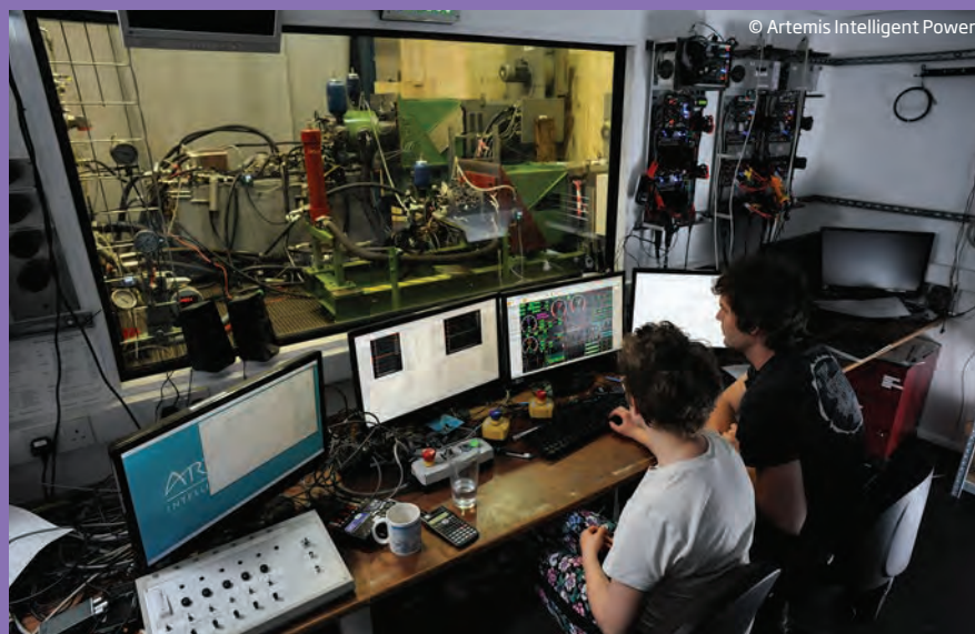
A member of the Artemis Intelligent Power team tests the performance of a 1.5 MW Digital Displacement motor
