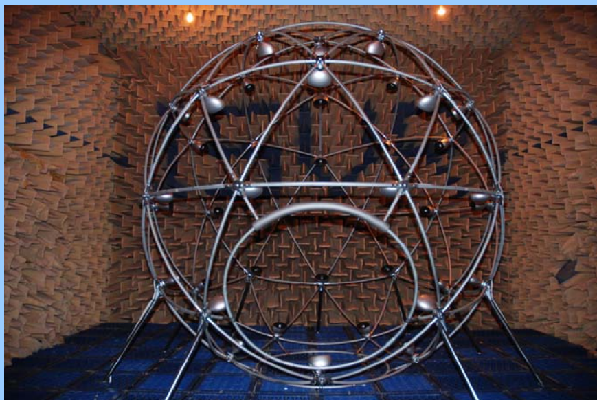
Experimental setup for ETRI-ISVR joint project on sound field reproduction. The support by ETRI of Korea for the experiments depicted above is gratefully acknowledged.
