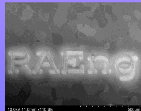
Fig.3. fs laser radiated graphene sheets on copper.
