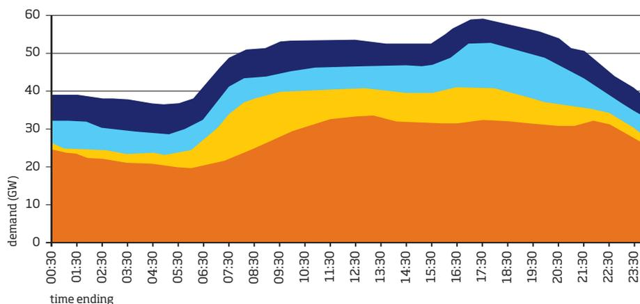
Figure 4.1 Typical demand profile of the GB electrical system<sup>32</sup>
