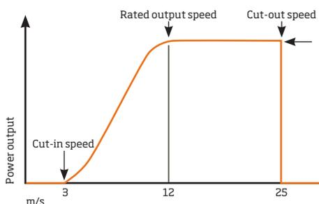
Figure 1.1 Typical wind turbine power output with steady windspeed
