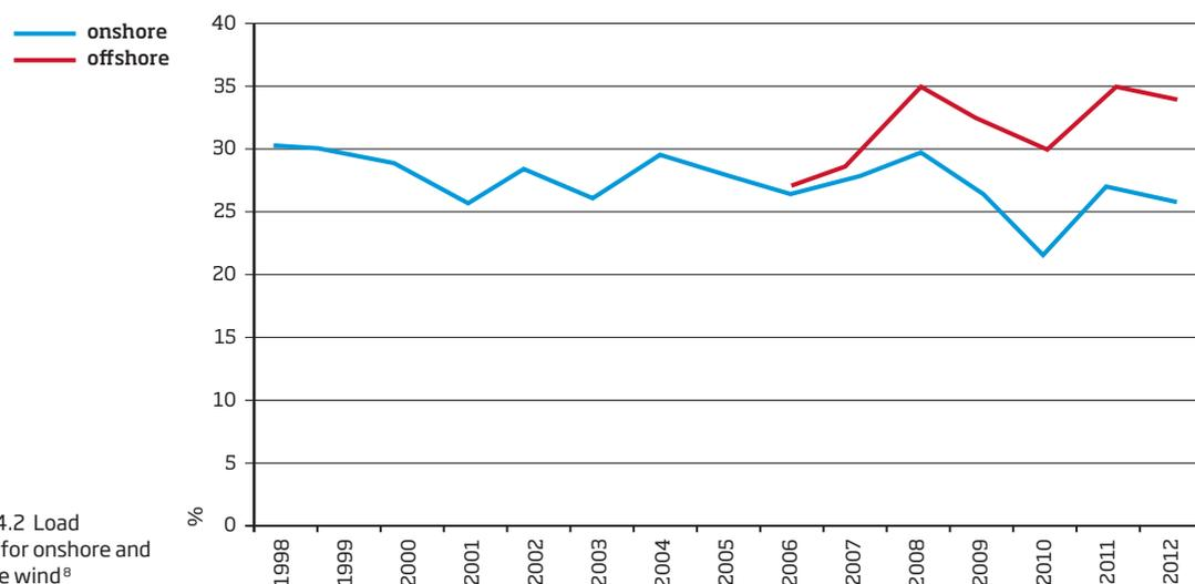
Figure 4.2 Load factors for onshore and offshore wind<sup>8</sup>
