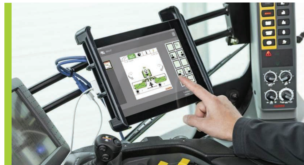
The Claas EASY on Board App was developed as a direct result of customer feedback. Connected by WiFi, a tablet can monitor, control and log data from equipment attached to the tractor © Claas
