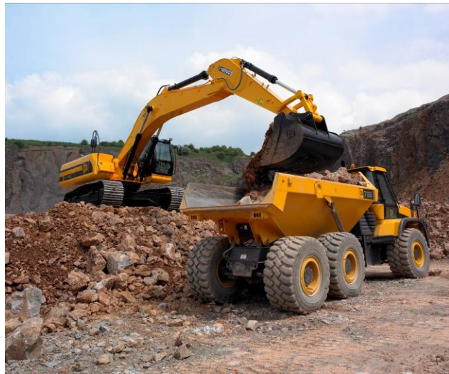
Figure-1: A JCB machinery loading rubble from a construction site into a truck
