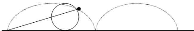
Figure 2: Locus of a point on the rim of the wheel for an observer on the ground
