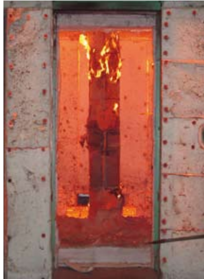
A full-scale structural fire test on a reinforced concrete column, strengthened with a fibre reinforced polymer wrap
